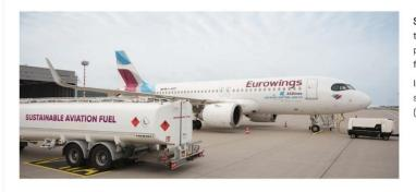
Sustainable aviation fuel (SAF) is the first realistic alternative to fossil aviation fuel . Compared to kerosene, SAF reduces additional CO  $_2$  emissions by at least 80%. An innovative production process reuses carbon from sustainable biomass and converts it into fuel. Only waste material from forestry and agriculture or used cooking oil is used for this process.
