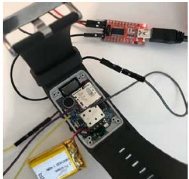
Figure 2. Assessing debug interfaces on the Tinitell.
