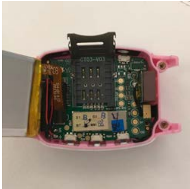
Figure 9. To install a SIM card in the Gator 2, you first have to disassemble the watch.
